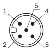
Connection diagram UM30-21x113 Connector M12, 5-pin
