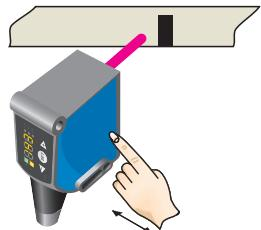
When setting the contrasts to be detected, "2nd" flashes. Press set button.
